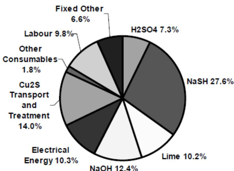
significant cost is that of the estimated transport and smelting/ refining charges applied to the  $\text{Cu}_2\text{S}$  precipitate, if sold to the local Enami copper smelter at Paipote near Copiapo, Chile.
