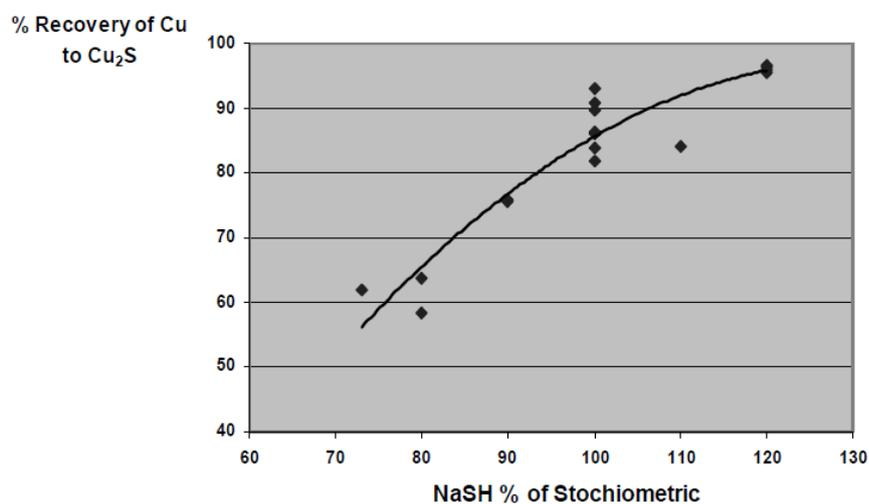
Figure 6 SART Cu Recovery As A Function Of % NaSH Addition Rate
