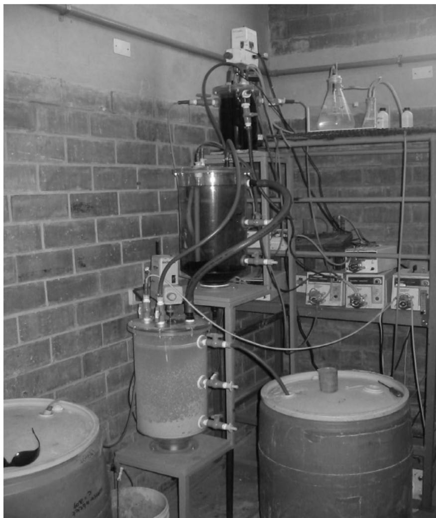
Figure 7 SART Pilot Plant Test Rig
